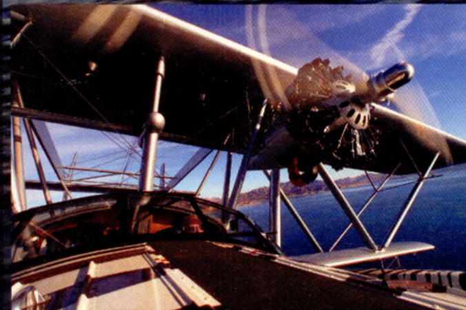
Engine cowlings were added to later Sikorsky seaplanes (below). Waldo Anderson (center) demonstrates a water takeoff before swapping seats with the author. The Pratt & Whitney engines are relatively close to the aircraft's centerline (right), which simplifies engine-out procedures.
